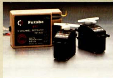
The 3S system sports two tiny S20 servos and a double-tuned, RF amplified 3 channel receiver.
